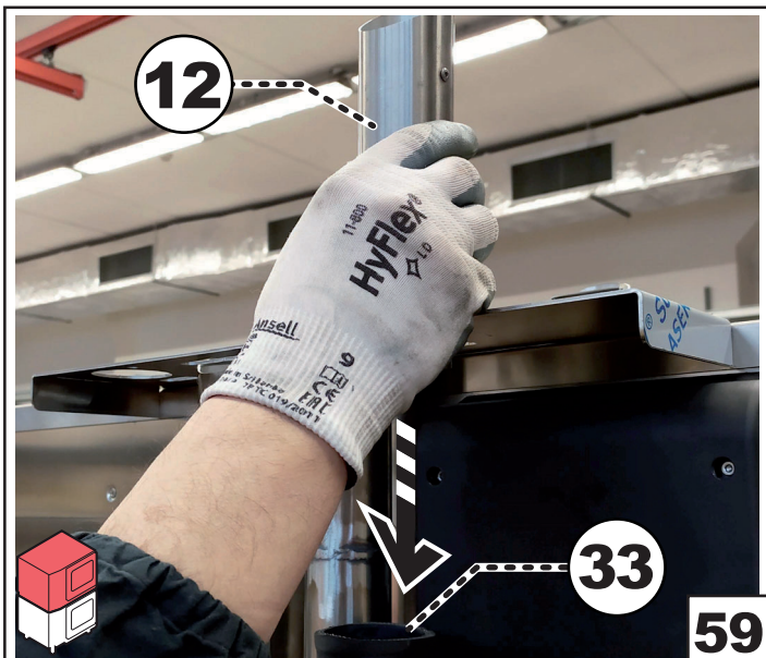
Insert the terminal tube in the extension rubber tube
