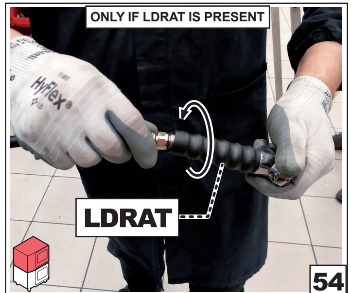
Fasten the nozzle of the LDRAT
