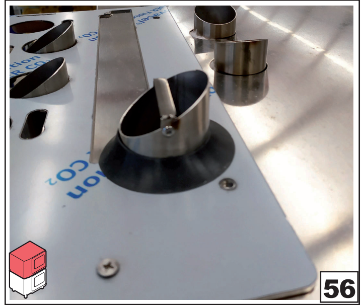
Be careful to place the tube gasket as in the image
