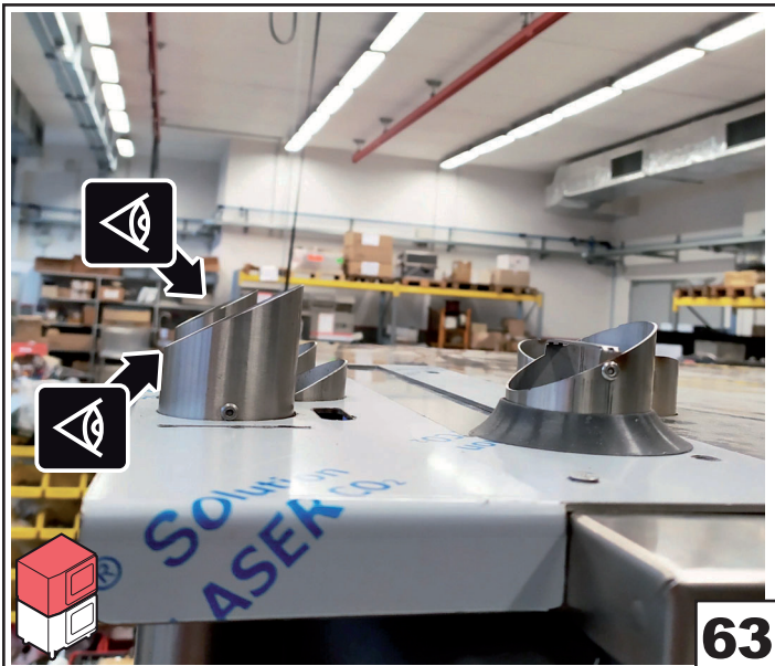
Be careful to check the direction of the last part of the tubes
