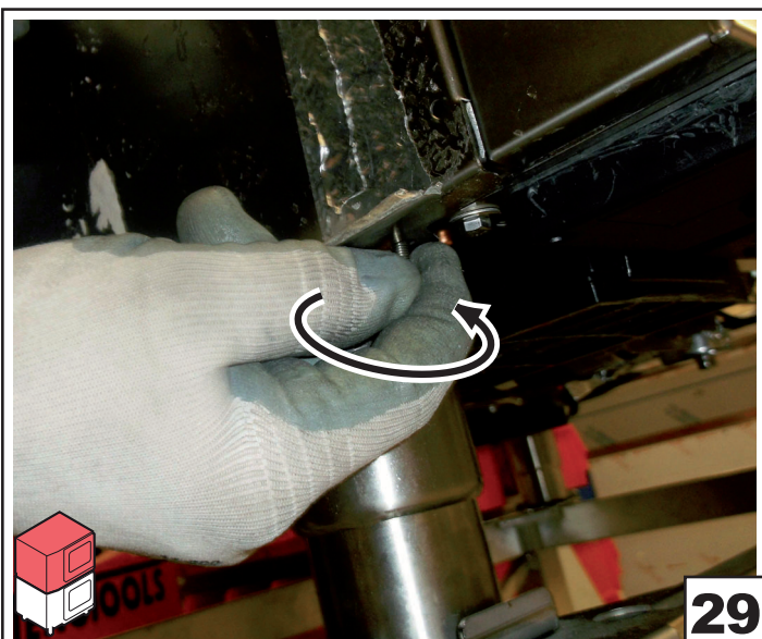
Remove the left side panel unscrewing the two screw placed on the bottom side
