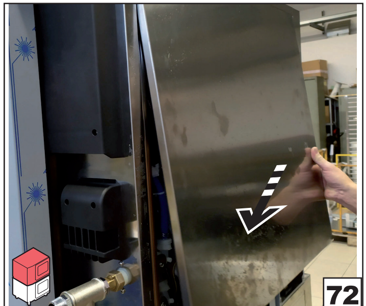
Place the left side panel of the upper oven
