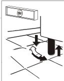
**WARNING:** If the appliance is not properly levelled the performance and condensate drain may be hampered.
