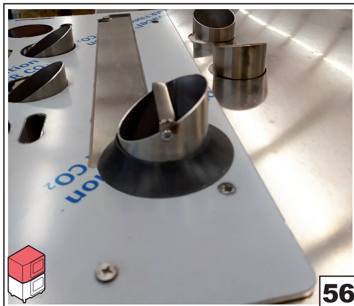
Be careful to place the tube gasket as in the image
