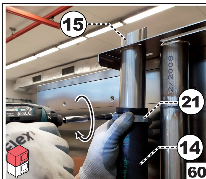
Tighten the metal clamps in the upper part
