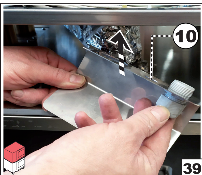
Fix the screw removed before in step 29 to lock the upper oven to the bottom oven
