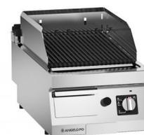
Grill range made of AISI 304 stainless steel, 20/10 mm thickness top. Cooking griddle made of enamelled cast iron with special nanotechnology surface treatment for a better fats sliding, delivered with stainless steel splash guards and cleaning brush. Heating by burner with thermocouple pilot light and piezo-electric ignition. Cooking takes place by irradiating ceramic elements heated by the burner.
