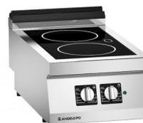
Electric range with pyroceram surface with AISI 304 stainless steel structure, 20/10 mm thickness top. Cooking surface in pyroceram, flush with worktop and sealed. Heating by infrared electric elements. 2 cooking independent areas controlled by energy regulator.
