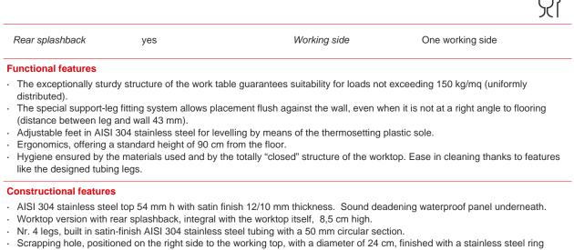
Scrapping hole, positioned on the right side to the working top, with a diameter of 24 cm, finished with a stainless steel ring
